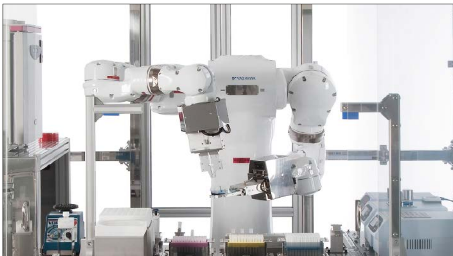
The MOTOMAN dual arm robot in a biomedical cell where it performs all the necessary tasks in a laboratory environment.
