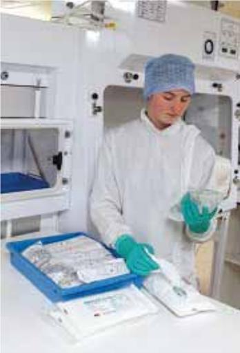
Figure 2: Presaturated sporicidal wipes are required in the UK for manual transfer disinfection.
