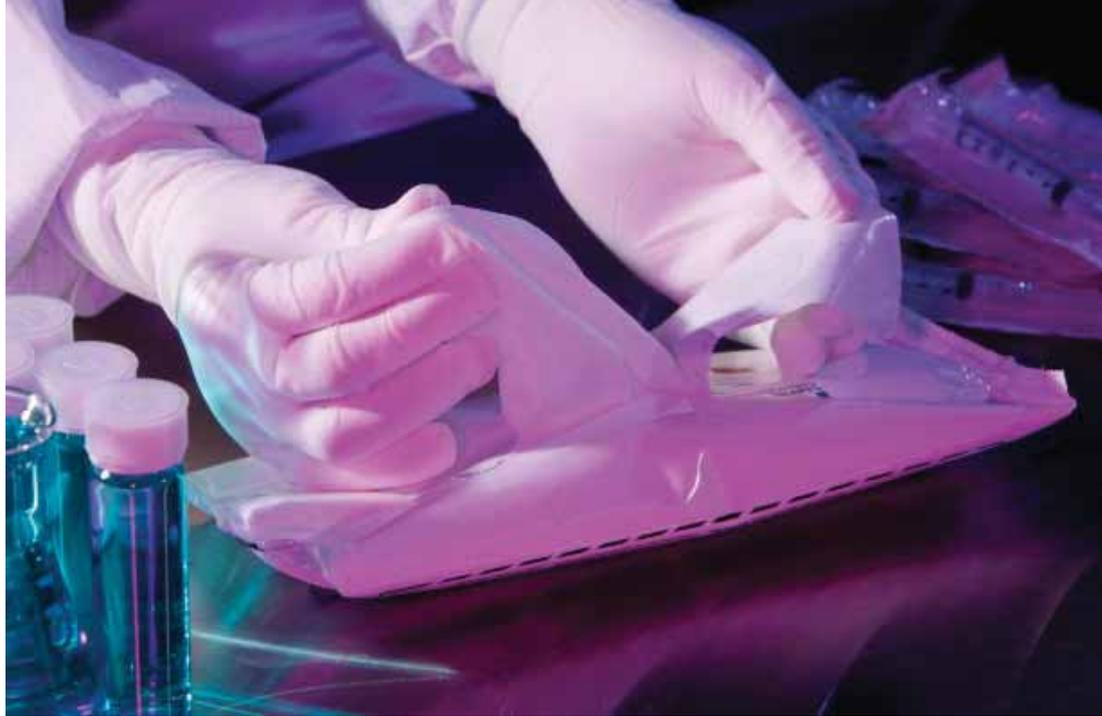
Figure 3: Resealable pouches are a convenient method of providing presaturated wipes for high grade areas.
