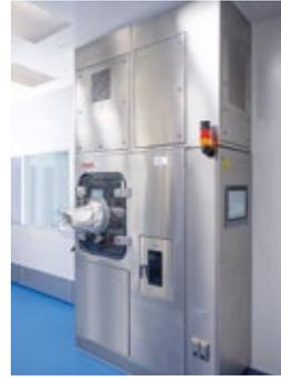
**Abb. 5: Stand-alone ISS H<sub>2</sub>O<sub>2</sub>-Transfer-schleuse**
