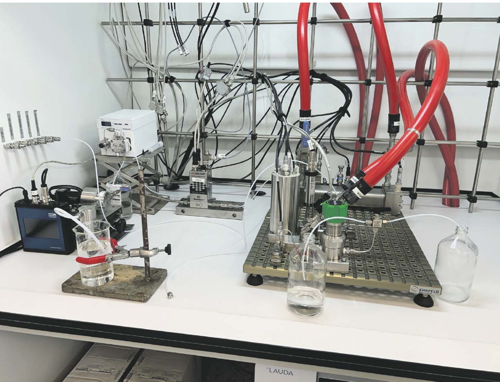
Fig. 1: Lab scale setup with a 30 mL reactor, two dosing units, sensors (mass flow, temperature, pressure) and connection to heating and cooling units.
