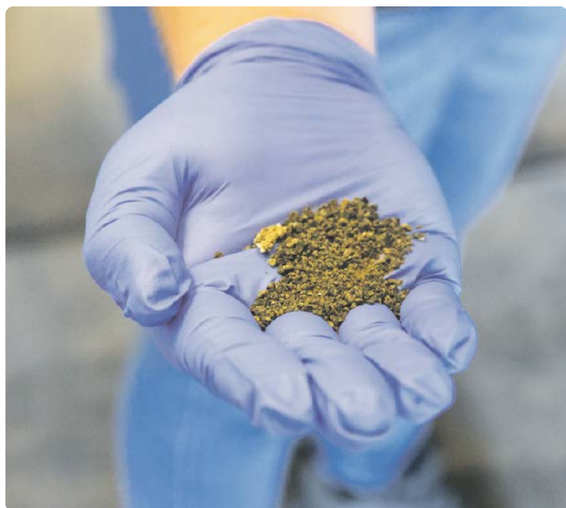
Green Li-ion's Green-hydrorejuvenation technology enables the generation of precursor cathode active material (pCAM) directly from black mass feedstock in under 12 hours.
