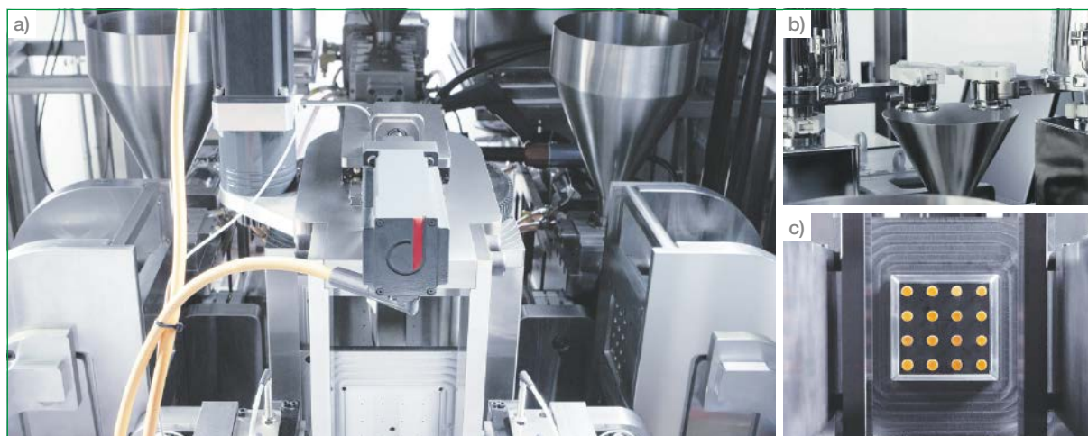
Fig. 2. Proprietary Continuous extrusion molding unit operation: a) main view, b) gravimetric feeders, and c) tablets in the mold.
