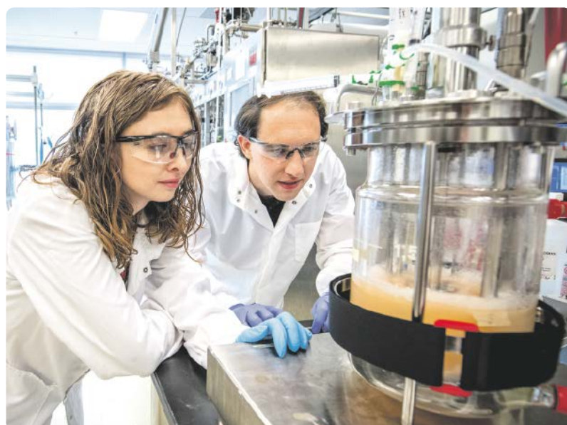
Microbial fermentation produces Aralez Bio’s enzymes which in turn make non-canonical amino acids.
