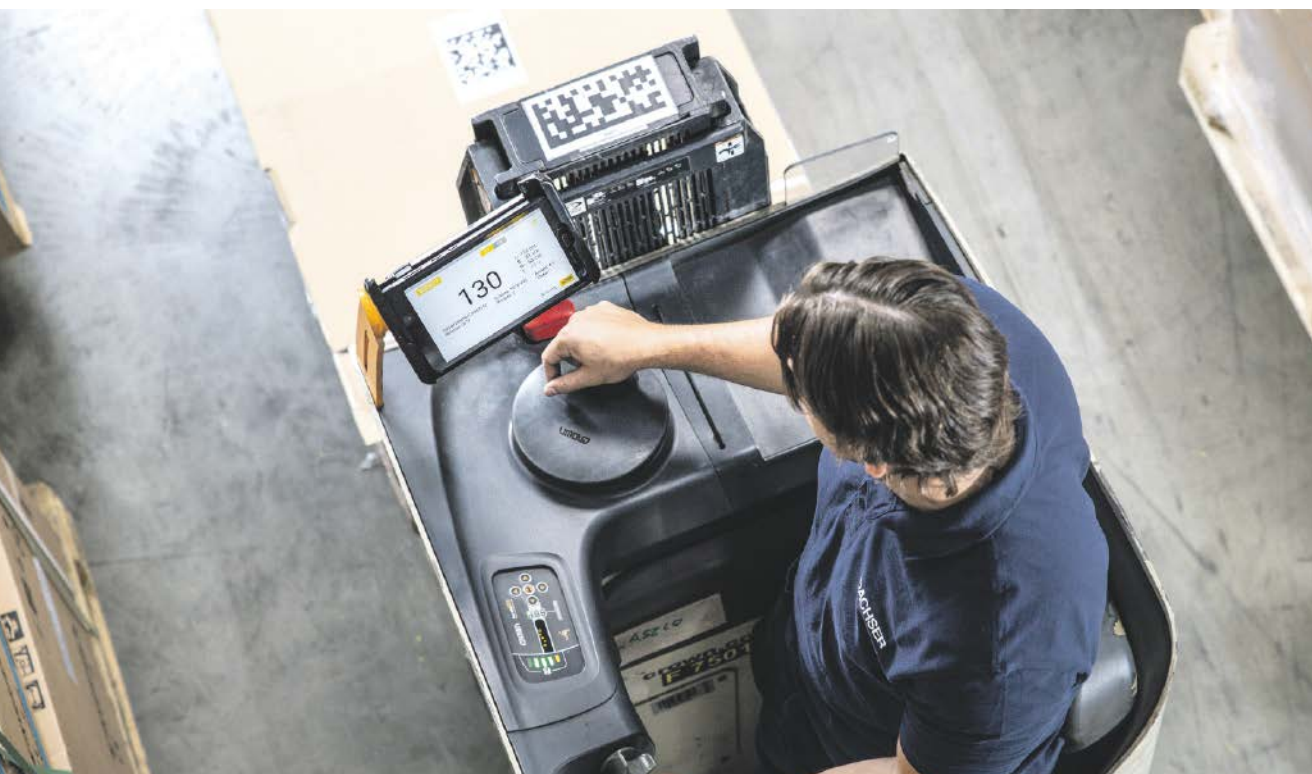
The information provided by Dachser's digital twin @ILO on displays and mobile devices can save forklift drivers and warehouse workers 15% to 35% off individual process times.
