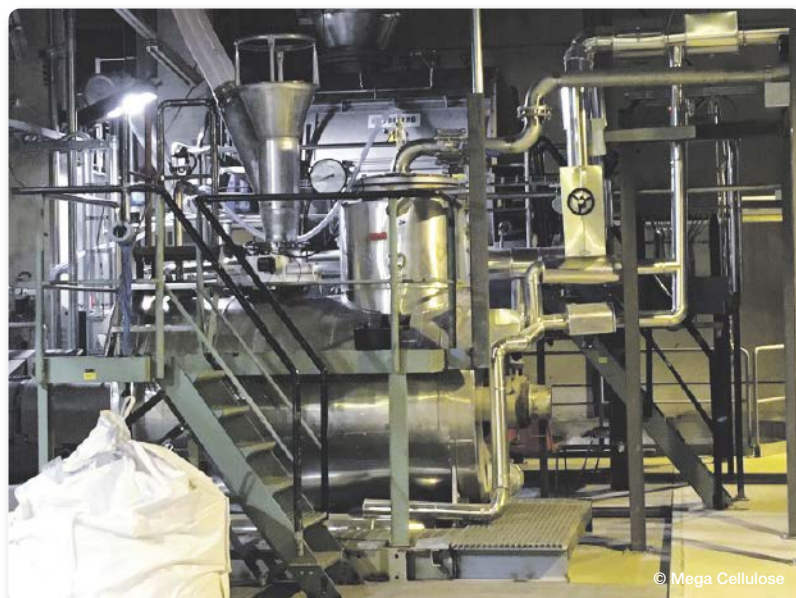
Mixed bulk reactors are particularly well suited for modification of natural polymers.
