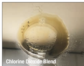
Figure 2: The build-up of residue of different cleanroom disinfectants on a surface. Mirrors were used to show residues more easily.
