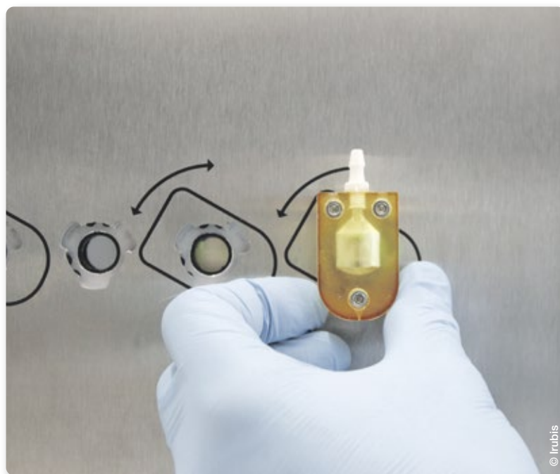
Single-use flow cell with silicon ATR crystal. It easily click-mounts to Monipa.
