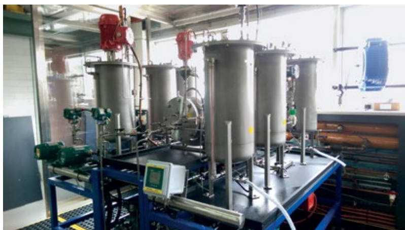
Fig. 2: A pilot scale tubular continuous flow reactor for manufacture of metal organic frameworks (MOFs) developed at CSIRO.
