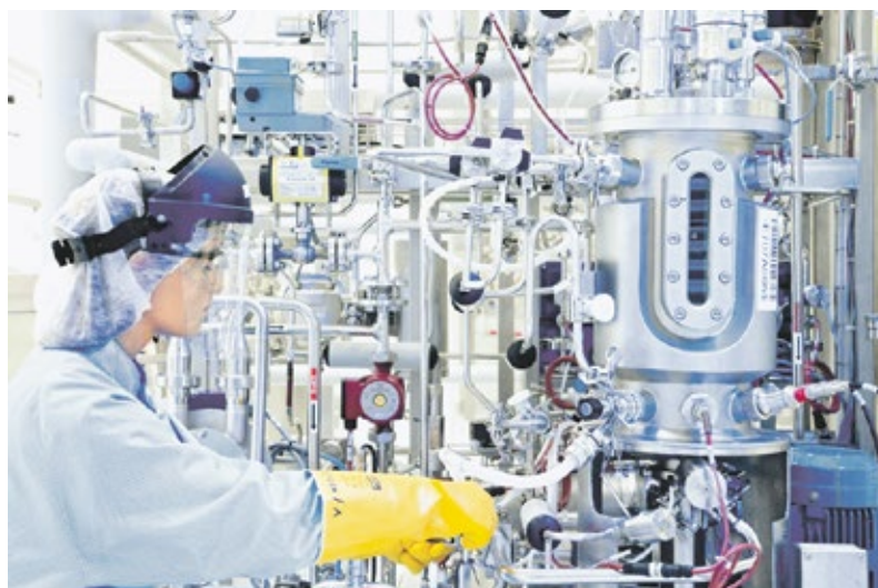
Sampling of the 15L pressed fermenter at Lonza BioPharma in Visp, Switzerland.
