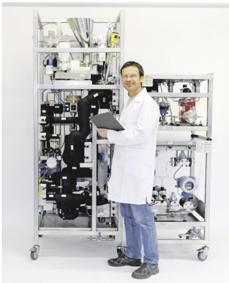
Fig. 1: Continuous cryogenic GMP plant for a liquid solid reaction.
