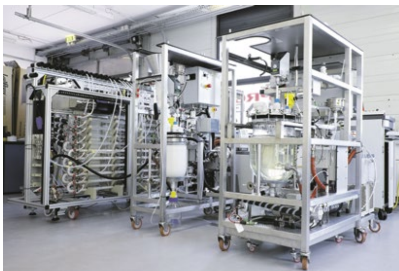
Fig. 2: Modular continuous crystallization plant for downstream processing.
