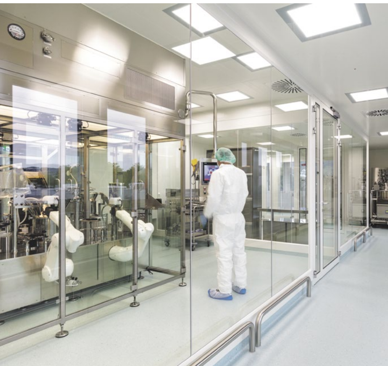
Vial-filling robot in sterile production area at the new compounding pharmacy of Kantonsapotheke Zürich, winner of the 2019 FOYA Operational Excellence Award Category.
