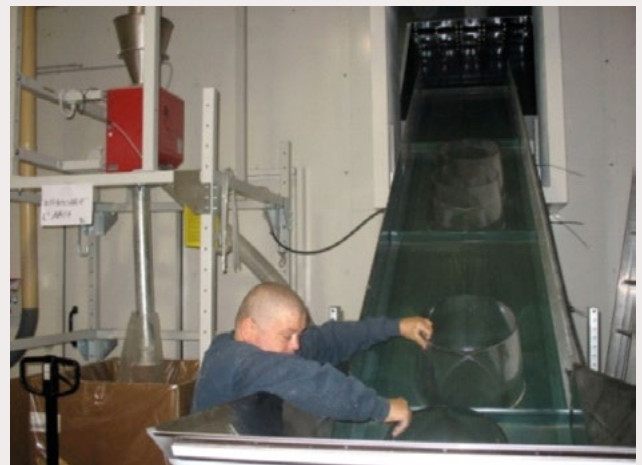
Fig. 2: A plastic Shredder machine which grinds the old plastic cages to offer a second life to the plastic material as automotive parts, furniture and other urban equipment.
