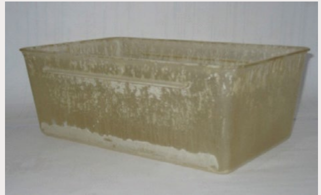
Fig. 1: A plastic cage at the end of its life cycle, unusable due to loss of transparency after many autoclave and wash cycles.
