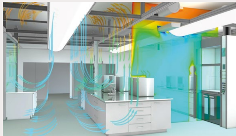
Fig. 3: Thermodynamics of supply air
