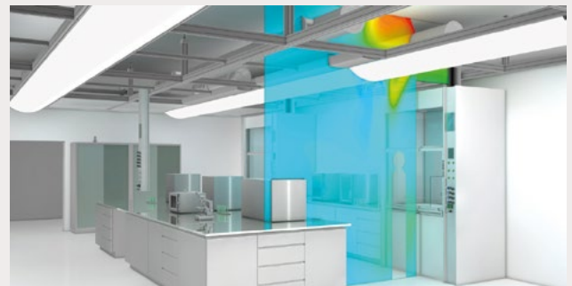
Fig. 5: Ventilation design of a lab
