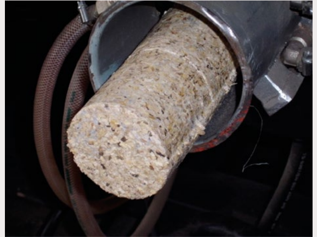
Fig. 4: Cage waste bedding now compacted as a briquette before disposal or incineration.
