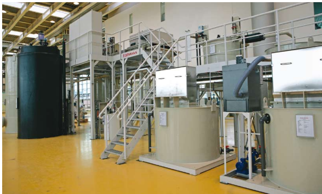
Fentox plant for purifying wastewater from the production of organic siloxanes
