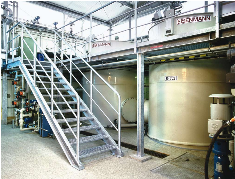
Fig. 3: Fentox plant for purifying seepage water from landfills on the site of a chemical park operator
