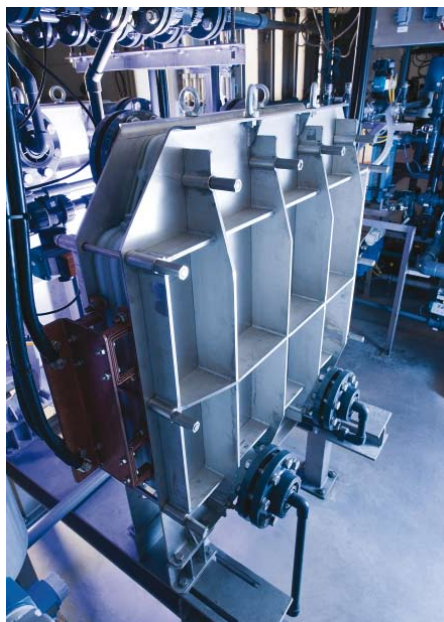
Fig 1: Electrolysis cell treating wastewater and producing hydrogen peroxide in situ
