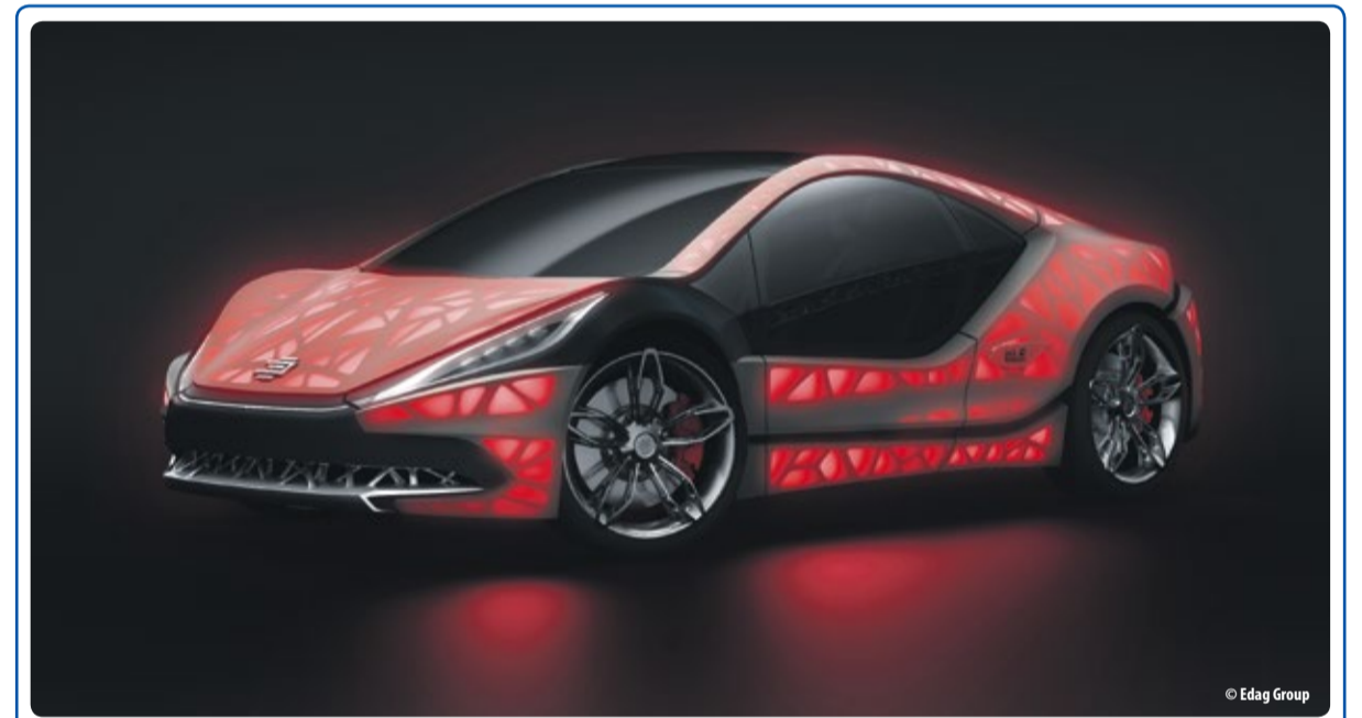
LED It Shine — German engineering firm Edag developed a concept car with a fully bionically optimised, additively manufactured (3D-printed) vehicle structure. The 'Light Cocoon' focuses on lightweight construction and to this end takes inspiration from nature. The concept features an organic-looking, lattice-like passenger cage covered with a weatherproof textile outer skin panel, produced by outdoor specialists Jack Wolfskin. LED lighting technology installed behind the outer skin panel makes the vehicle's skeleton-like structure visible. The color of the outer skin can be changed at will, according to the driver's taste. Despite the fact that material has only been used in areas where it was necessary for function, safety and stiffness, all requirements imposed on structurally relevant components are met. (rk)
