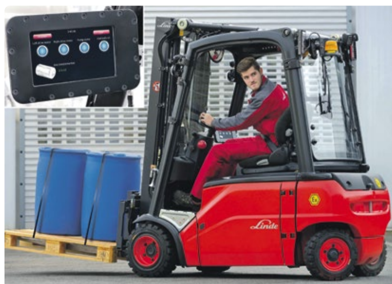
The radio-controlled gas warning system from French specialists Centrexpert is available as an option for Linde electric forklift trucks used in explosion-protection zone 2 with a load capacity of between 1.4 and 3.5 tons. Source: Linde Material Handling, Aschaffenburg, Germany
