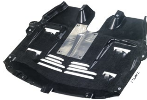
Fig. 2: The engine compartment guard plate shows that Tepex dynalite has great potential for use in underbody protection for cars – particularly for cars destined for countries where road conditions are generally poor.
