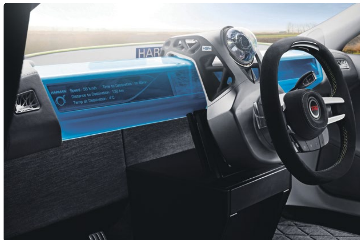
In the XchangeE concept car, it consists of a 1.2-meter-wide display strip made of Plexiglas LED in the steering wheel support. This strip is also transparent when unlit, and can change color when lit. In both cases, a clear view of the instrument panel is provided.
