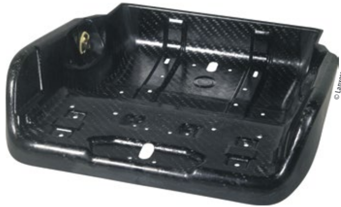
Fig. 1: Despite its thin walls, the seat shell is very rigid and strong. In the event of a crash, it absorbs more energy than comparable designs such as those made of plastics reinforced with long glass fibers.
