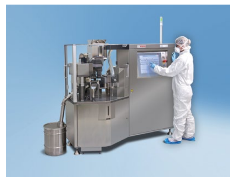
Bosch's KX 3900 simultaneously inspects process quality parameters such as weight, length and condition of filled capsules
