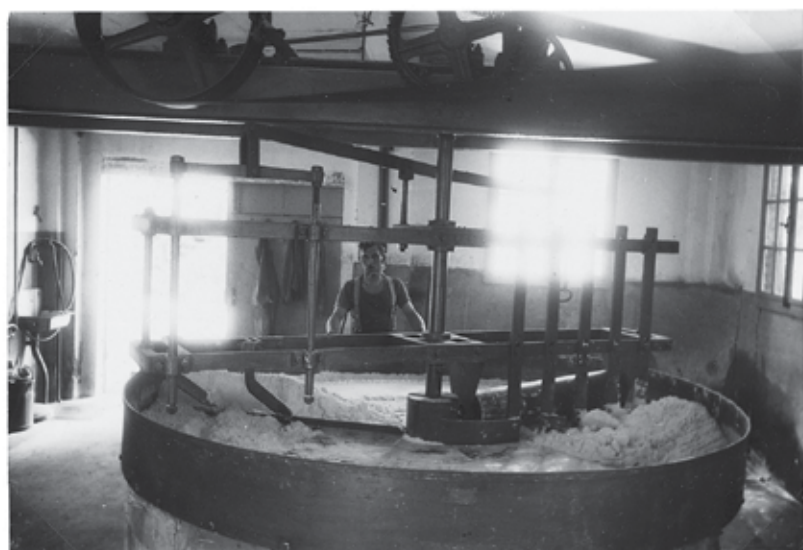
Ammonium nitrate drying trough in the beginning of Schweizerische Sprengstoff-Fabrik AG (SSF) in Dottikon
