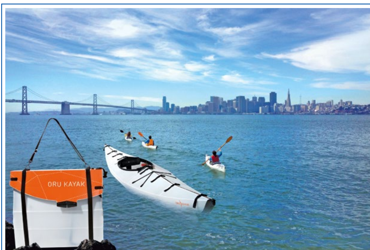
Origami Boat - The Oru Kayak is a high-performance boat that folds out of a compact case. Its designer Anton Willis — inspired by origami — began creating this folding kayak after a move into a small San Francisco apartment forced his fiberglass kayak into storage. The full-size (12' long), and super light (25 lbs) Oru Kayak is engineered of a single sheet of double-layered plastic that is extremely tough and durable. The single seam is sealed with a watertight rubber gasket. Solid ribs offer strength and rigidity. On the water it's fast, stable and handles well. Folded and stowed in the case it can be stashed in a trunk, checked on a plane or even carried on a hike to remote waters. (Photo: www.orukayak.com)
