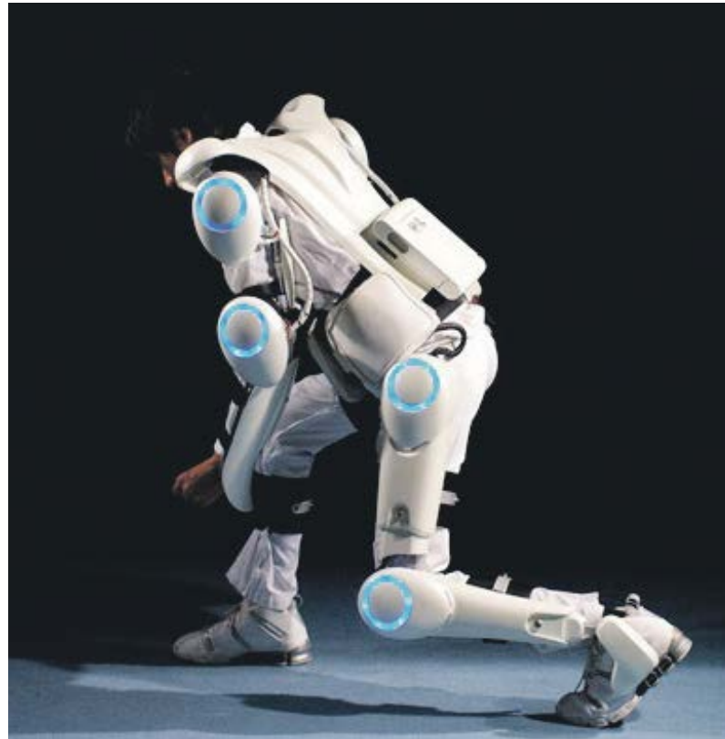
As part of the cooperation with Japanese professor Yoshiyuki Sankai, a renowned expert in exoskeletal robotic systems, BMS is contributing an extremely lightweight, super strong reinforced polycarbonate material to Sankai's much-touted Hybrid Assisted Limbs (HAL) therapeutic program.
