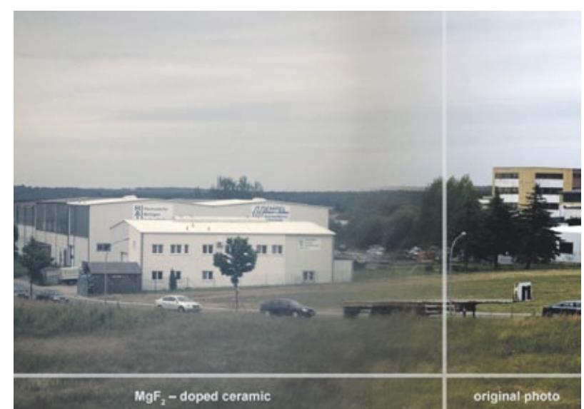
Figs. 1a and 1b: Plane glass surface coated with a hard, transparent MgF 2 -layer. The small zone on the right side of the surface shows the original, non-coated glass area.
