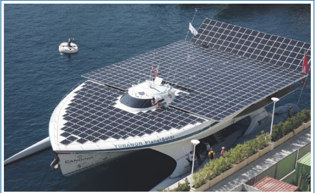
Power of the Sun – The stunning catamaran PlanetSolar that has been launched in March 2010 in Kiel, Germany, is the winner of the 2012 Practical Boat Owner (PBO) Green Award for having circumnavigated the globe using solar energy only. DuPont, an official partner of PlanetSolar, has supplied Tedlar polyvinyl fluoride (PVF) film, which is used as a component for the photovoltaic backsheets. It helps protect the modules and ensure reliable power generation and avoid any energy source failure. The biggest solar run ship in the world exposes to the sun a total of 537 m 2 of photovoltaic surface with a panel efficiency of 18.8% that powers a 6-block lithium-ion battery.
