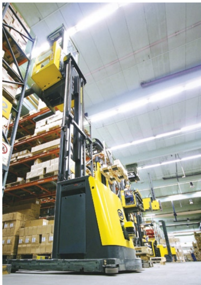
Five XOP2 vertical order pickers in man up version equipped with additional fork lengths for comfortable picking.
