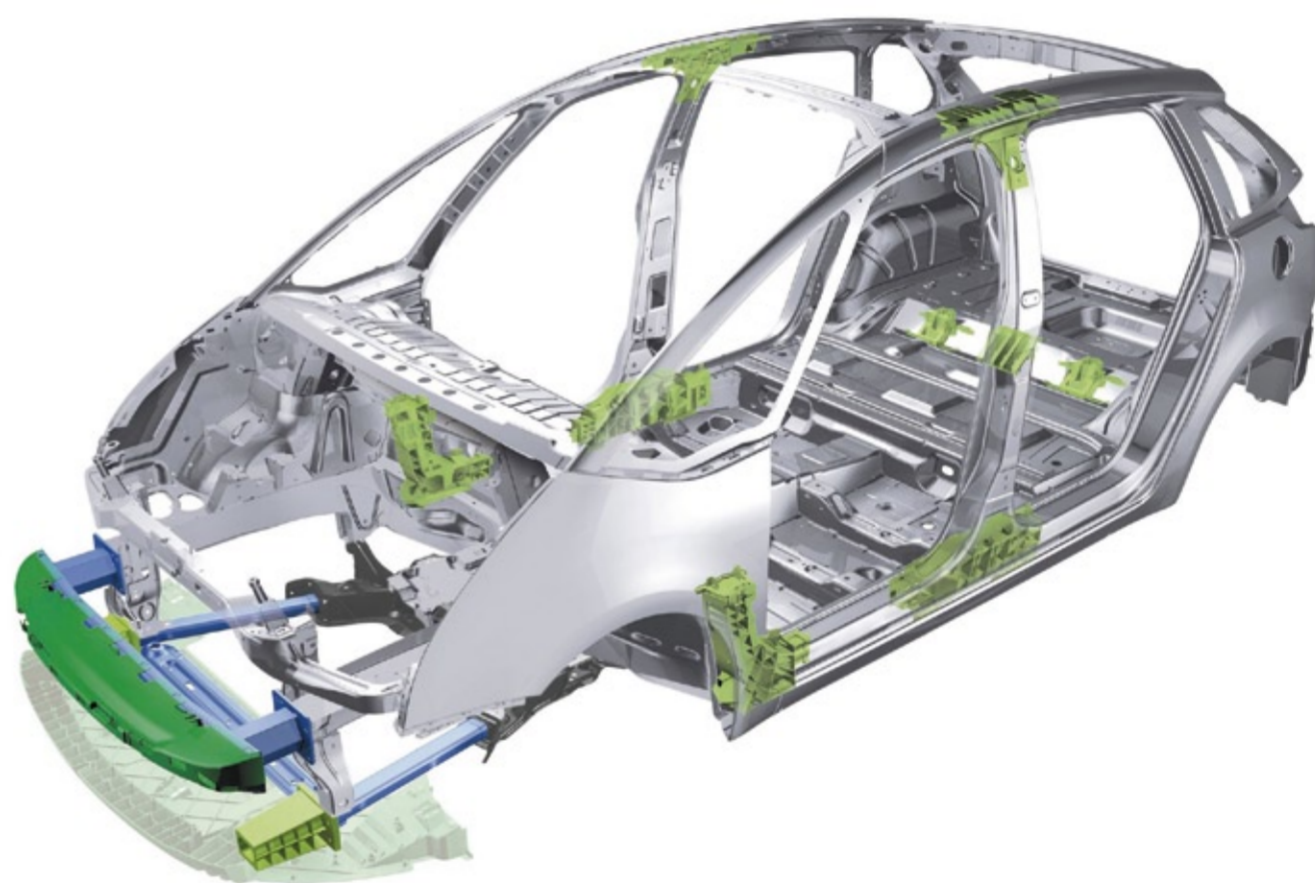
Fig. 1: The structure inserts are fitted deliberately in crash-relevant areas of the body and are located in the lower part of the A pillar, in the lower and upper part of the B pillar and in the transverse beam above the rear axle. (Photo: Citroën)
