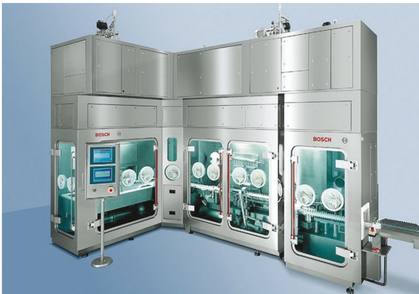
Bosch has further developed the FLM 4080 filling and closing machine and now offers it with a bio-decontamination module integrated in the isolator. The module generates hydrogen peroxide steam using a process which operates more simply and reliably than previous procedures and also provides very short sterilization cycle times.
