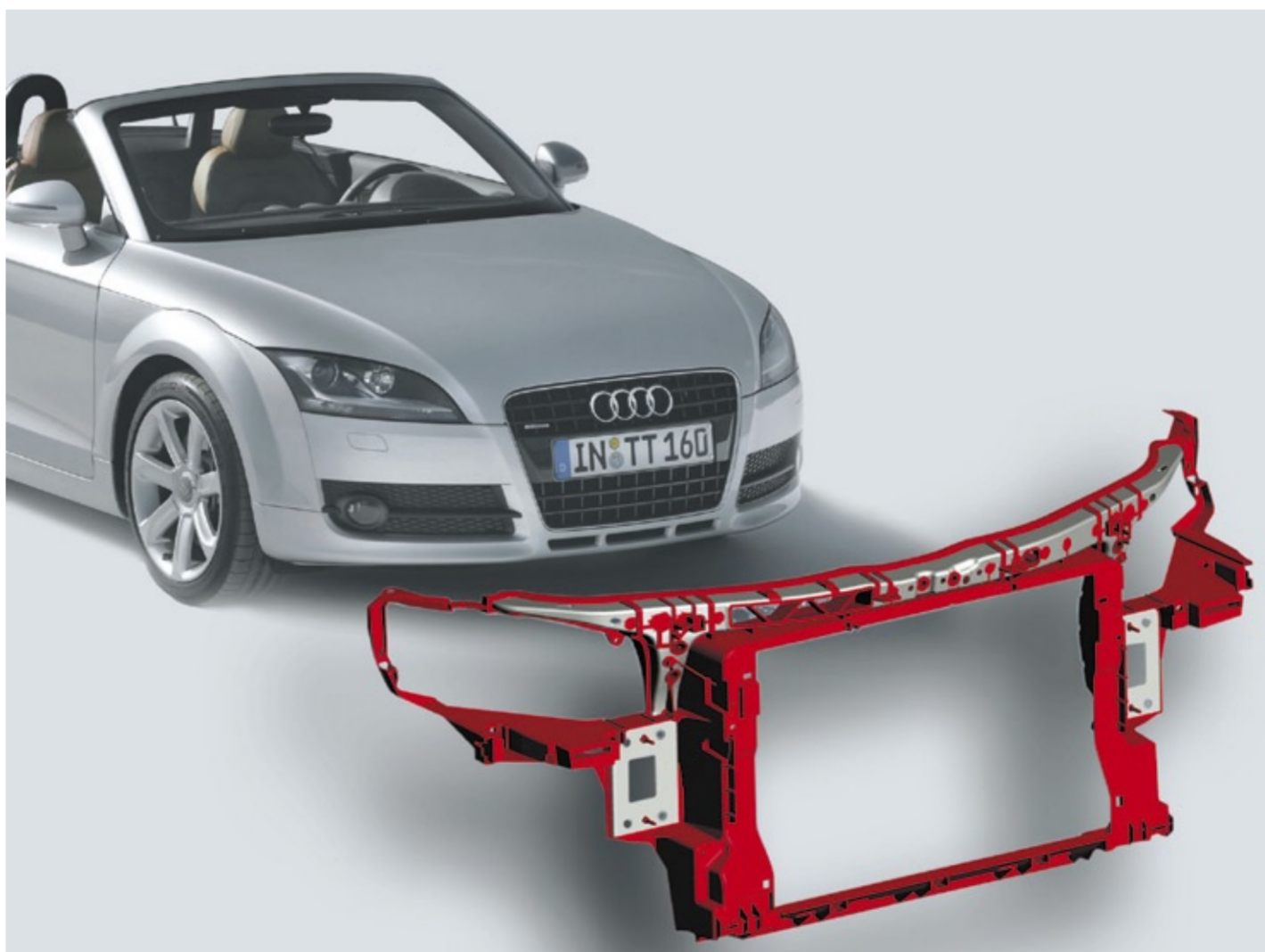
Fig. 2: In the Audi TT, the first front end in plastic aluminium composite structure is on the road. It is made up of three aluminium sheets spray-coated with polyamide 6 Durethan BKV 30. (Photo: Lanxess)
