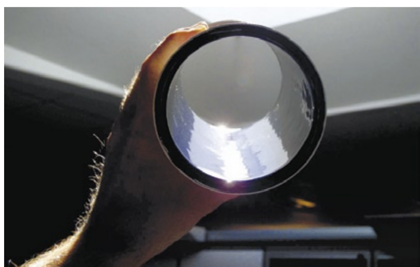
Glasslined technical equipment with extremely smooth surface finish in conjunction with high wear resistance to abrasive acting media and high resistance to corrosion. Visual counter light inspection of surface.
