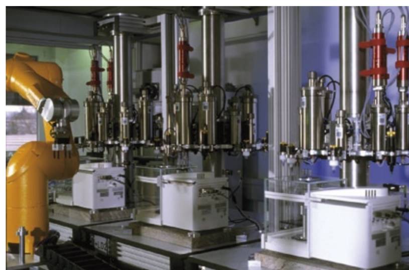
Figure 2: Partial view of a high-throughput formulations platform, showing the articulated arm robot on linear track and the viscous fluids dispensing stations.
