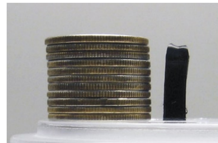
Researchers at the University of Cincinnati have grown the world's longest carbon nanotube arrays, long enough to be seen by the naked eye.
