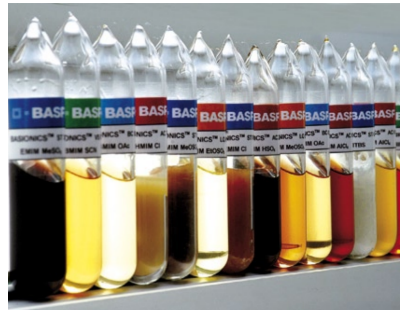
Ionic liquids: phase separation in the BASIL process, above the product and below the ionic liquid. Using this process, the scavenging of an acid with a base results in a liquid salt instead of solid crystals that can cause problems in large-scale production. With so-called ionic liquids, time-consuming and expensive filtration is no longer necessary.
