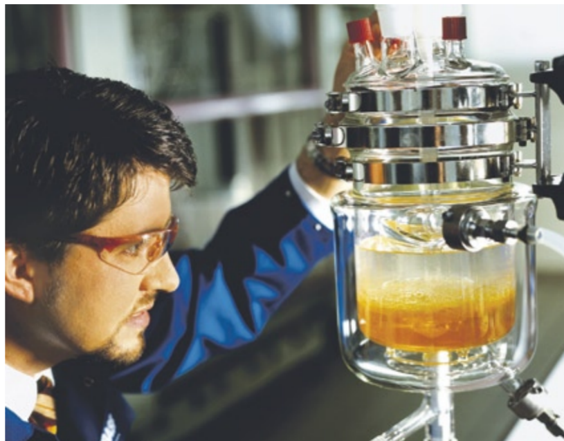
Ionic liquids: phase separation in the BASIL process, above the product and below the ionic liquid. Using this process, the scavenging of an acid with a base results in a liquid salt instead of solid crystals that can cause problems in large-scale production. With so-called ionic liquids, time-consuming and expensive filtration is no longer necessary.
