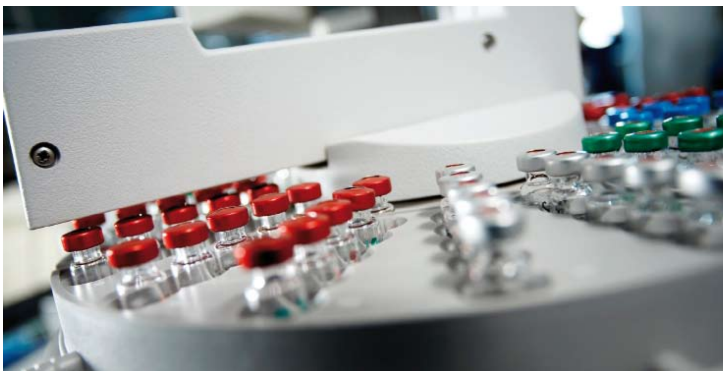
CATALYST DEVELOPMENT: Gas chromatography is used to separate the product of a catalytic reaction into its individual components and to analyse whether the catalyst employed has produced the desired chemical product. Photo: BASF
