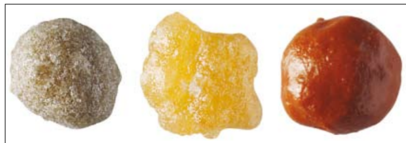
Product examples, from left to right: spray granulation enzyme – spray cooling lipid coating – spray granulation beta carotene
