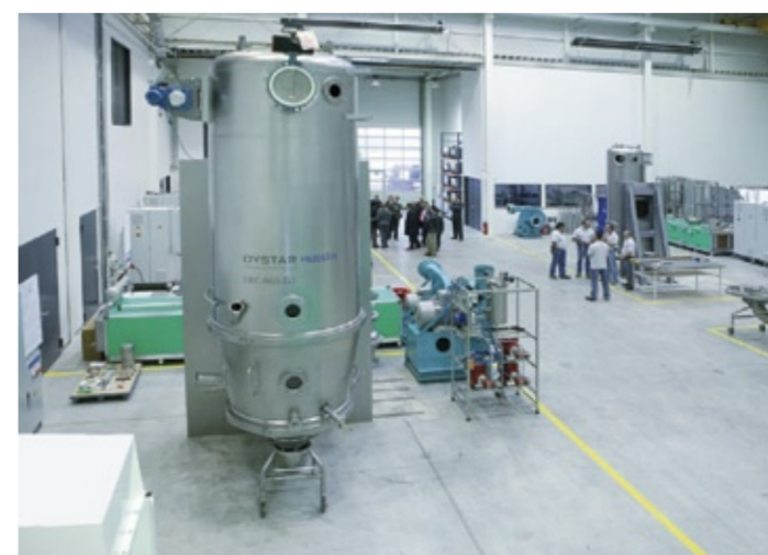
HKC 600 DJ, a fluidized-bed equipment for granulation, drying and coating in Oystar Hüttlin's production hall.
