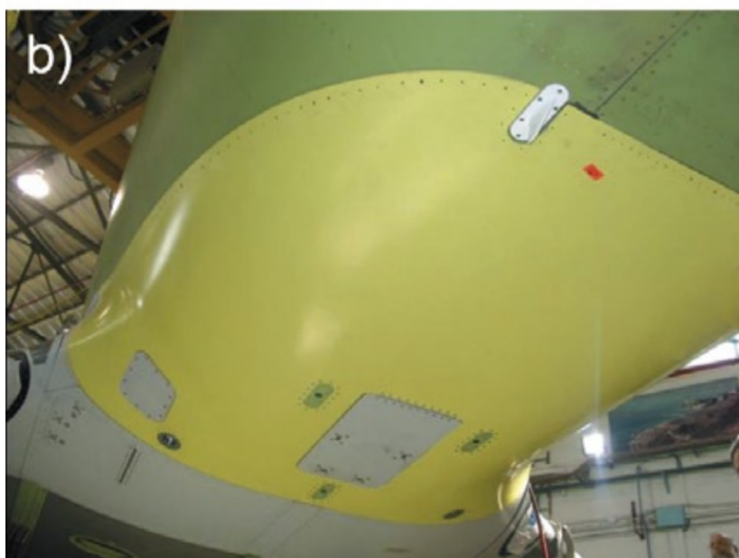
One of the two Rohacell cores. b) Assembled Gulfstream G 150 belly panel.
