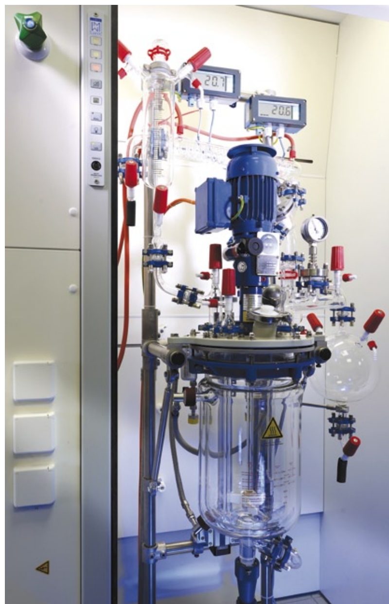
10 L scale-up reactor
