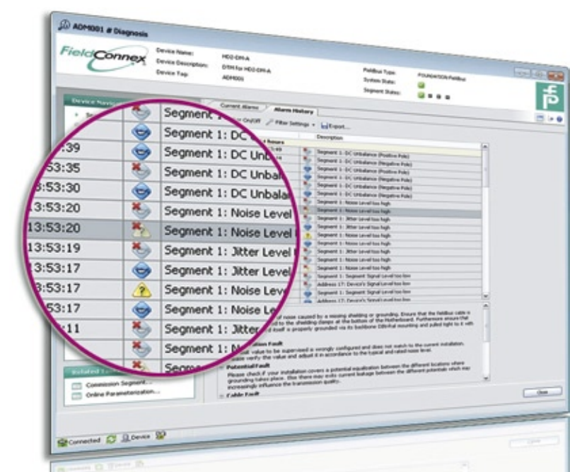
Physical layer diagnostic display: Messages with time stamps and clear-text interpretation identify potential causes – powered by the built-in expert system.
